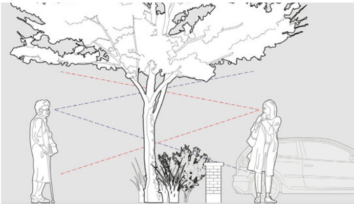
An open field of view at eye level promotes observation and safety
