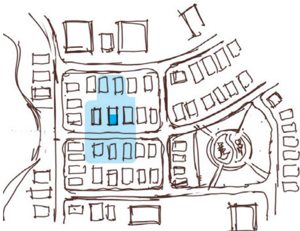
The area of influence for modifications to an existing site or building will generally be the immediate neighbouring and facing properties.
